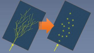
Fast simulation: a full shower is replaced by a parametrized version of it
